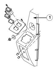
8. Locate the old shroud locking bracket behind the new shroud (1). Replace the old shroud locking bracket with the new locking bracket (2).
