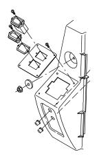
7. Disconnect, remove, and set aside the on/off key switch, scrub switch, and circuit breakers from the right hand side of the shroud. (Refer to FIG. 1)
