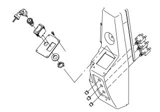
8. Remove the hex screw and nut holding the squeegee lift handle to the fixed steering housing. Let the handle drop down off the housing. Set the handle aside. (Refer to FIG. 1)
