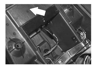
4. All of the electrical components that are contained in the instrument panel and on the electrical mount panel, can now be easily accessed. Label all accessory wires before disconnecting from accessories mounted in the shroud. Cut and remove the plastic wire ties that are holding the potentiometer wire to the main panel harness.
