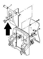
6. Disconnect, remove and set aside the hourmeter, battery discharge indicator and circuit breakers from the left hand side of the shroud. (Refer to FIG. 1)
