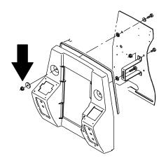
3. Tilt the instrument panel assembly back until it is resting against the lanyard strap.
