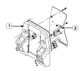
9. Slide the adjustable steering housing into the slots in the new housing (1). Reinstall the shroud adjustment knob and connect to the new locking bracket. Tighten the knob to secure the adjustable housing. Reconnect the stop switch to the wire harness. Reconnect the potentiometer to the controller. Secure the potentiometer wire to the main panel harness with the plastic wire ties (4).
