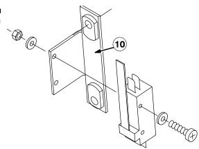
4. Mount the new switch bracket (10), squeegee pivot plate (14), and catch bracket (7) with hex screw (13), and mounting hardware from the old housing. Secure the side of the squeegee pivot plate (14) with the two rivets (15).
