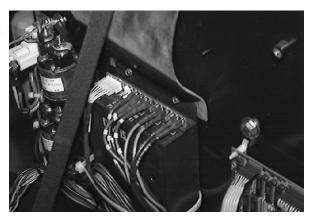
5. Unplug the potentiometer from the controller. Unplug the wire harness from the stop switch. Loosen the speed control handle latch, and remove the shroud locking bracket from behind the shroud. Set the locking bracket aside. Slide the adjustable steering housing out of the slots in the fixed steering housing. (Refer to FIG. 1)
