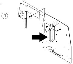
3. Remove the fan switch and mounting hardware from the old housing. Mount the fan switch to the new fan switch bracket (10) with mounting hardware.
