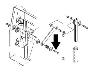
9. Disconnect the housing from the lanyard strap. Remove and discard the fixed steering housing. (Refer to FIG. 1)
