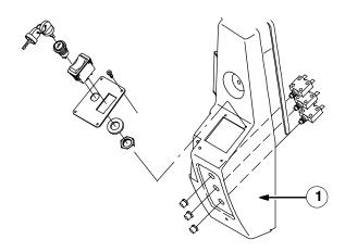
7. Install and reconnect the hourmeter, battery discharge indicator and circuit breakers on the left hand side of the shroud (1).
