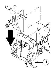
10. Install the two new hose hanger clips to the left hand side of the new housing (1) with hex screws (17), flat washers (18) and lock nuts (19). Hang the recovery and solution tank drain hoses back up on the hose hanger clips.
